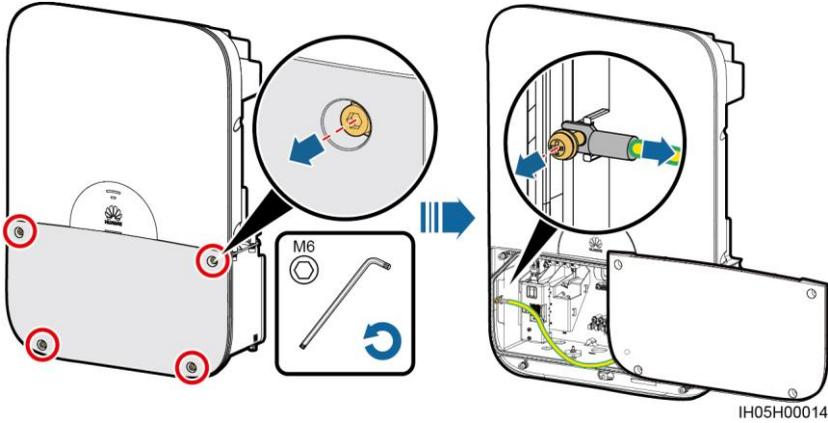
2. Removing the 10-pin signal terminal.
