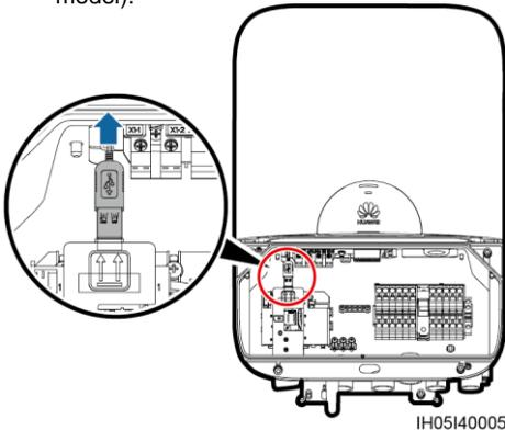
5. Removing the WLAN cable (only for the WLAN model).
