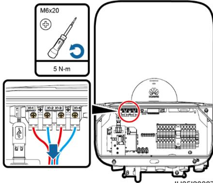
7. Remove the AC cable and the fuse cable.
