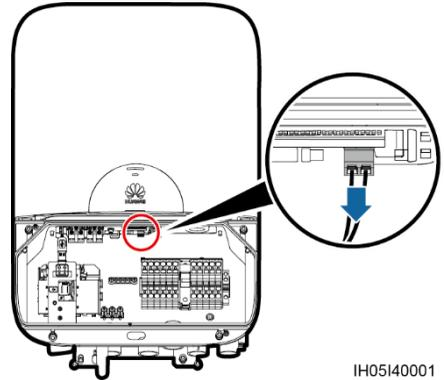
4. Removing the USB cable (only for the 4G model).
