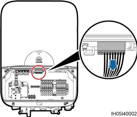
3. Removing the 2-pin enable terminal.
